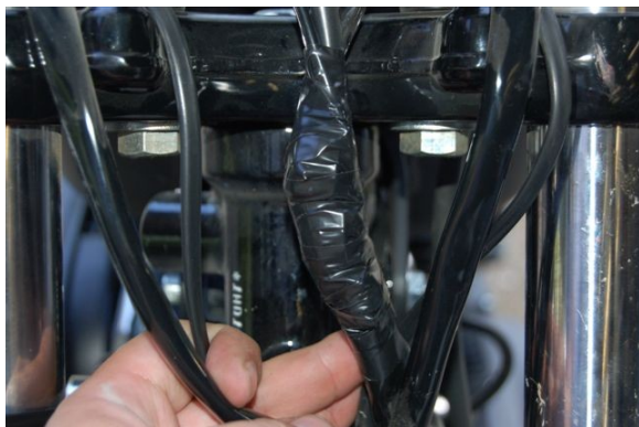
Figure 9: Tape bundle to seal out moisture
