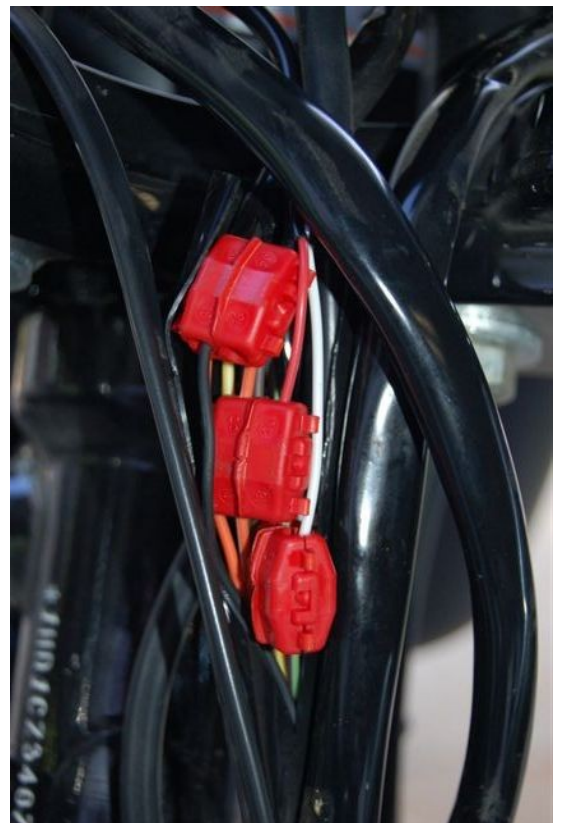
Figure 8: Stagger connectors to make smaller bundle size
